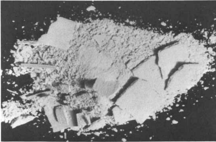
Figure 30. 1100 aluminum after four hours in distilled water at 315°C (22)
