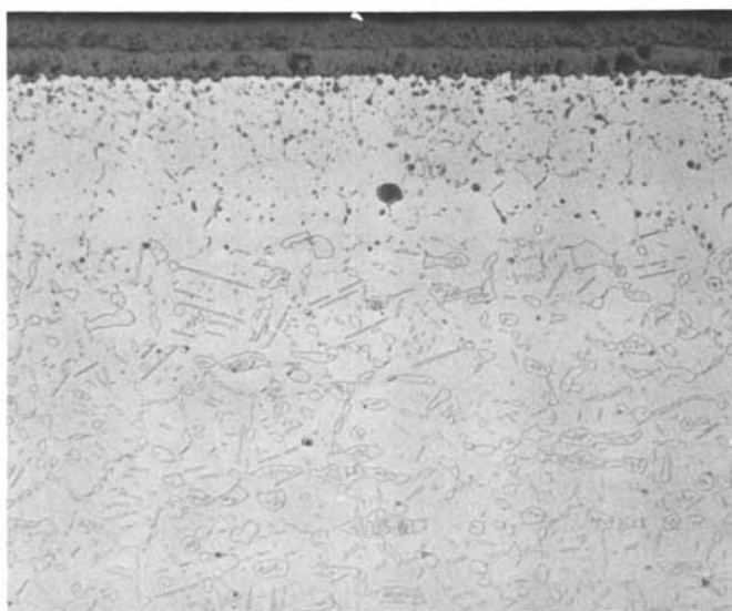
Figure 5. Surface microstructure of IN-671 after 5000-hour exposure at 1800°F in CGA gas containing 0.5 v/o H_2S . Neg. No. 44911 (170 \times ).
