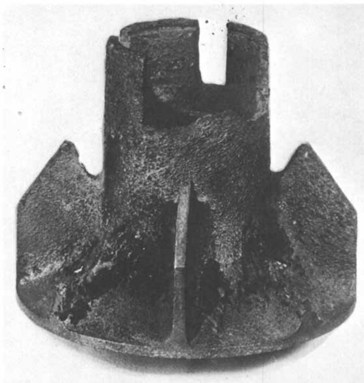
Figure 15. Cast-iron pump impeller with cavitation corrosion damage
